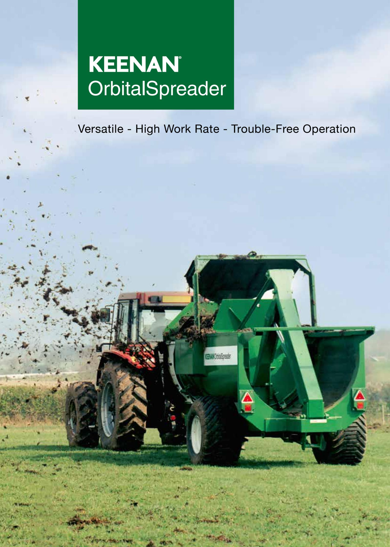
**The KEENAN® OrbitalSpreader is a heavy-duty versatile spreader. It is capable of very high work rates with trouble-free operation. Able to handle a wide range of farm and commercial wastes, it delivers a remarkably uniform spread pattern.**
